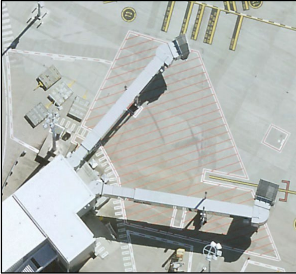
Figure 22 Red Hatching Lines – Safety Areas
