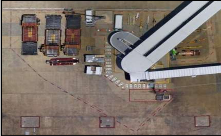
Figure 18 Single Broken Red Line - Staging / Clearance
