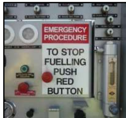
Figure 8 Emergency stop on vehicle
