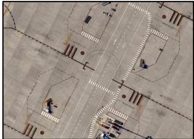
Figure 19 Both Staging and Storage Markings
