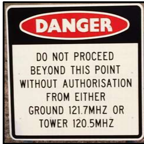
Figure 43 Taxiway Entry Warning Sign
