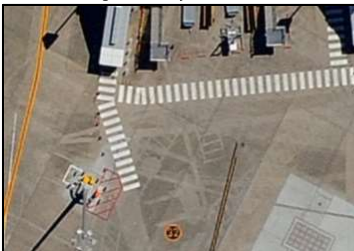
Figure 5 Pedestrian walkway and hatched eye wash station
