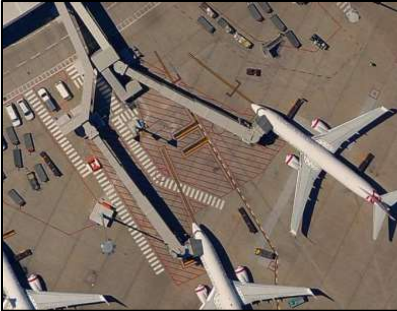
Figure 21 Red Hatching Lines - Safety Areas
