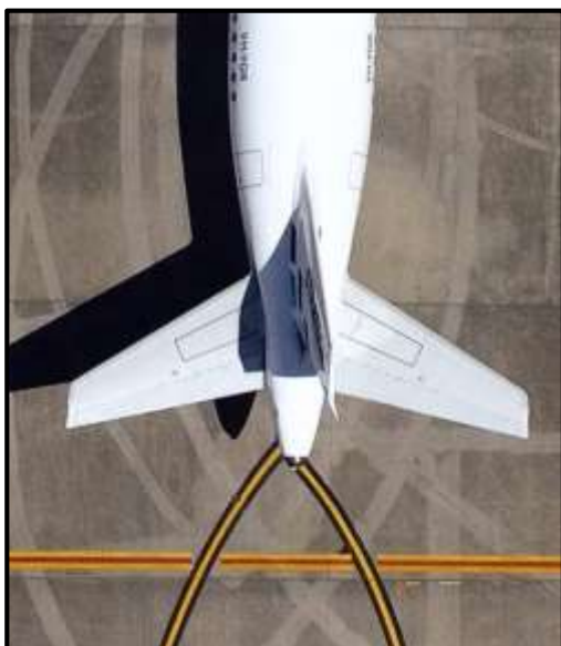
Figure 46 Parking Clearance Line
