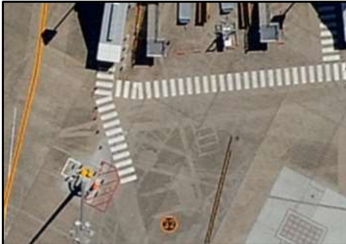
Figure 5 Pedestrian walkway and hatched eye wash station
