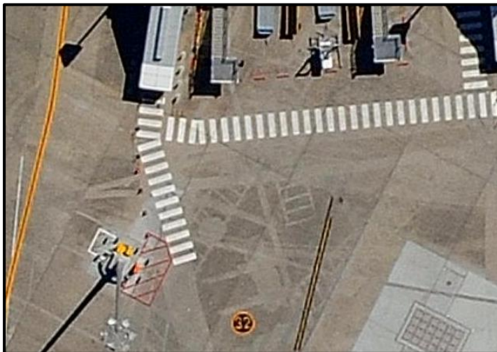
Figure 5 Pedestrian walkway and hatched eye wash station
