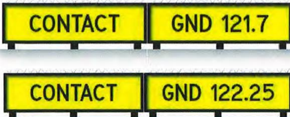
Figure 49 – Ground Frequency MAG Signs
