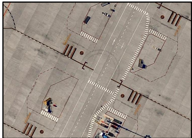
Figure 19 Both Staging and Storage Markings
