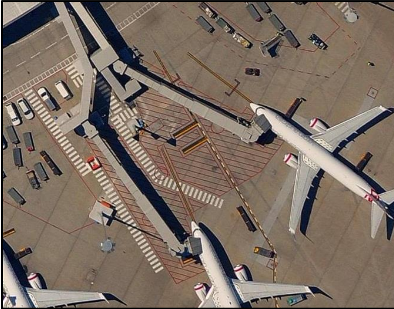
Figure 21 Red Hatching Lines - Safety Areas
